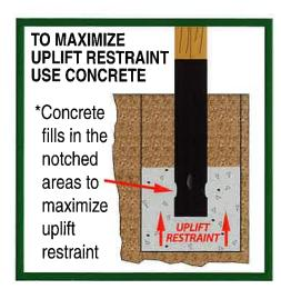
The Most Affordable, All-In-One Solution for Eliminating In-Ground Post Decay and Rot with Uplift Restraint
